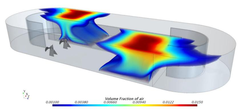
One of the most challenging applications of aeration in biological reactors are the so called oxidation ditches in wastewater treatment plants. Oxidation ditches are closed loop reactors equipped usually with fine bubble diffusers and large-diameter slowly rotating propellers. Goals of the process are the complete nitrification, nitrogen removal and also the prevention of sludge settling.
