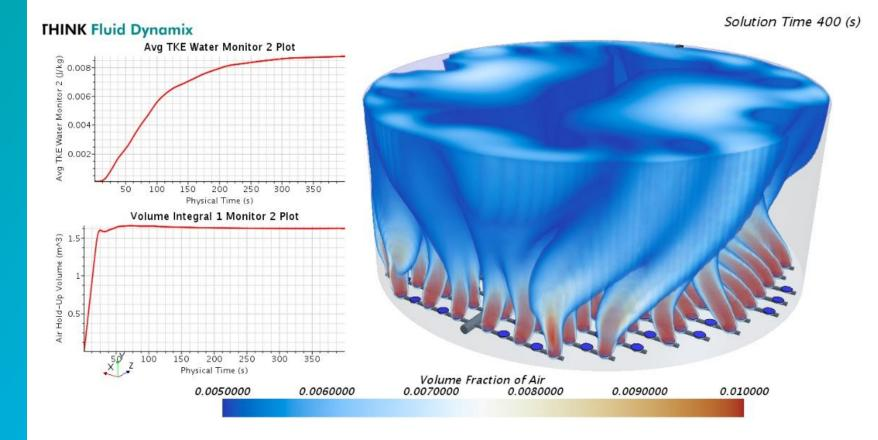
Fine bubble aeration is the best way to enhance the contact surface between the gas and the liquid phase resulting on higher mass transfer rate. There are, however, many other design parameters that has an influence on the oxygen transfer efficiency, for example the layout of the diffusers. With numerical simulations different designs can be analyzed to maximize design parameters.
