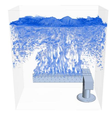
For many applications fine bubble diffusers cannot be installed or they perform with a poor efficiency, in such cases coarse bubble aerators have to be installed. Furthermore, coarse bubble aeration system are a good solution to add turbulence and mixing into the system. CFD simulations can provide an insightful description of such designs.
