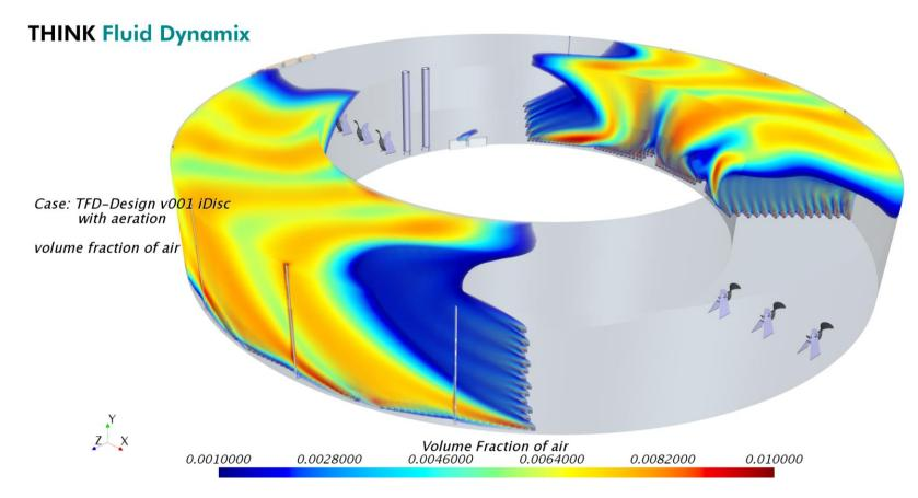
Oxidation diches exist in a large variety of shapes and sizes. This makes it very difficult to find general rules of thumbs to make efficient designs and therefore each case has to be specifically analyzed and , if necessary, optimized with the support of CFD simulations.
