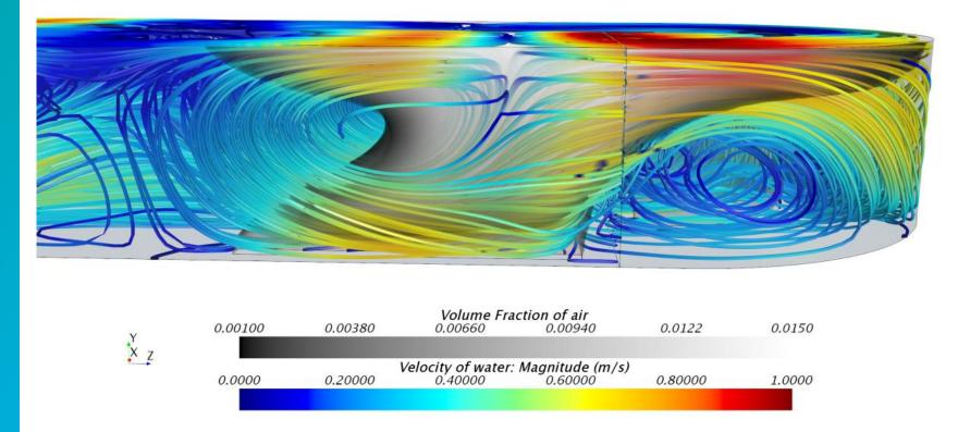
In oxidation ditches a natural conflict occurs between circulation flow induced by propellers and vertical flow induced by the buoyancy forces of the air load. A high air superficial velocity can result in the formation of strong vortex structures, which break the flow circulation and accelerate the natural rise of bubbles, resulting in a poor oxygen transfer rate and hence, in a lower reactor performance.
